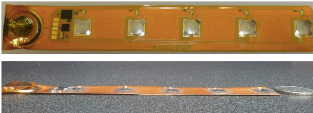
Figure 2. PosterVote: Flexible hardware to be placed at the back of each poster (the five buttons and the LEDs on top). In total, the hardware consists of a memory, a clock, five buttons, five LEDs, a placeholder for the battery and a port to download the results by using an FTDI to USB cable.
