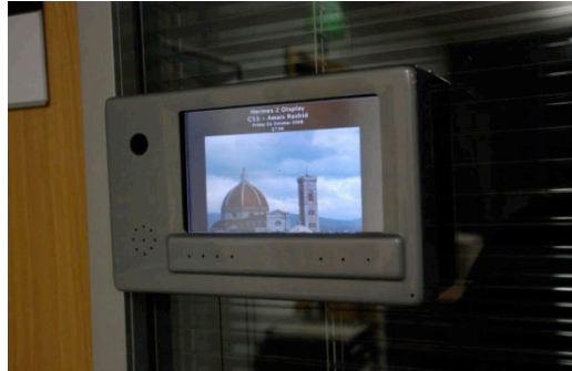
Fig. 6. A Hermes 2 display showing the owner message only, in this case the owner has chosen not to have his door display support the functionality enabling visitors to leave messages.
